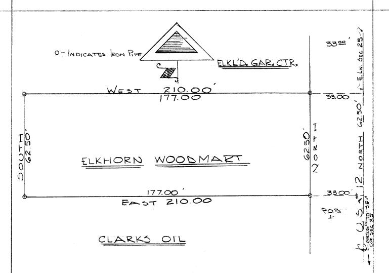
DESCRIPTION: Communing at a point in the East line of Section 25, T. 3 N., R.16 E. which is 635.60 feet North of the S.E. corner of said Section, thence North 62.50 feet to a point, thence Nest 210.00 feet to a point, thence South 62.50 feet to a point, thence East 210.00 feet to the place of beginning.
